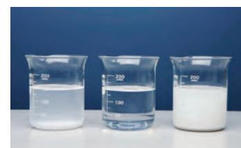
After settling for 20 minutes, the cup of water with PANACAL L- Calcium Lactate remains clear while white residue can be seen at the bottom of the other 2 cups.
